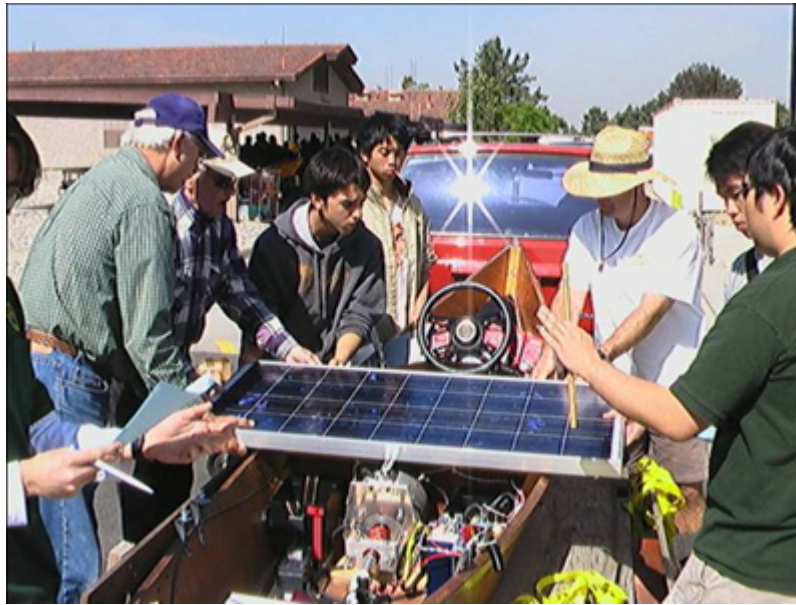
The Sharp 80W Watt solar modules both powered the boat and charged its batteries.
